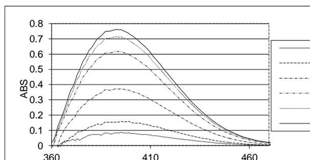
**Figure 2. Changes of the absorption spectra of the complex in ethanol at  $5 \times 10^{-4} \text{ M}$  due to the addition of various amounts of fluoride.**
